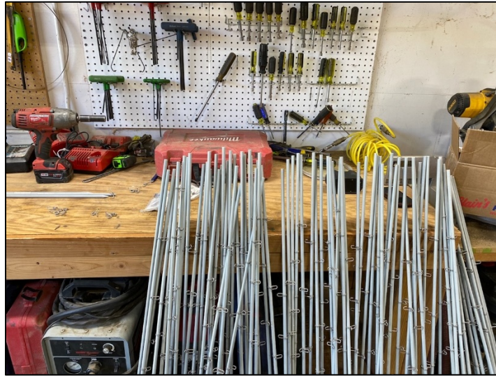
Fiberglass fence stays being outfitted with metal clips for wire attachment
