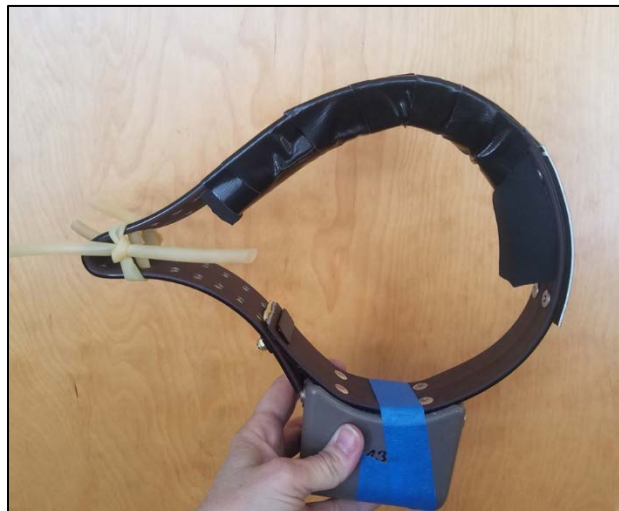
GPS collars modified to allow for neck growth for bighorn rams
